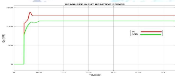
Figure 8: Simulation Waveform for Reactive powers of ES system with PI and ANN Controller Case 2: RCD control technique for Electric Spring with Conventional PI controller and ANN controller
