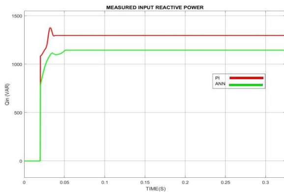
Figure 16: Simulation Waveform for measured Reactive Power of ES System with PI and ANN Controller.
