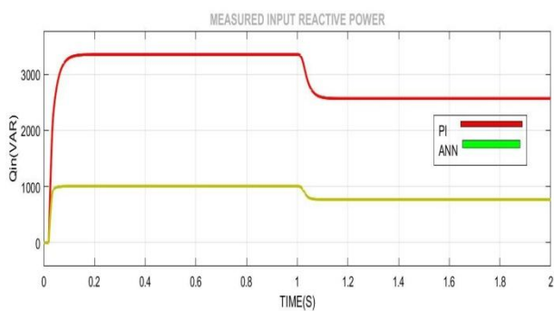
Figure 14: Simulation Waveform for measured Reactive Power of ES System with PI and ANN Controller
