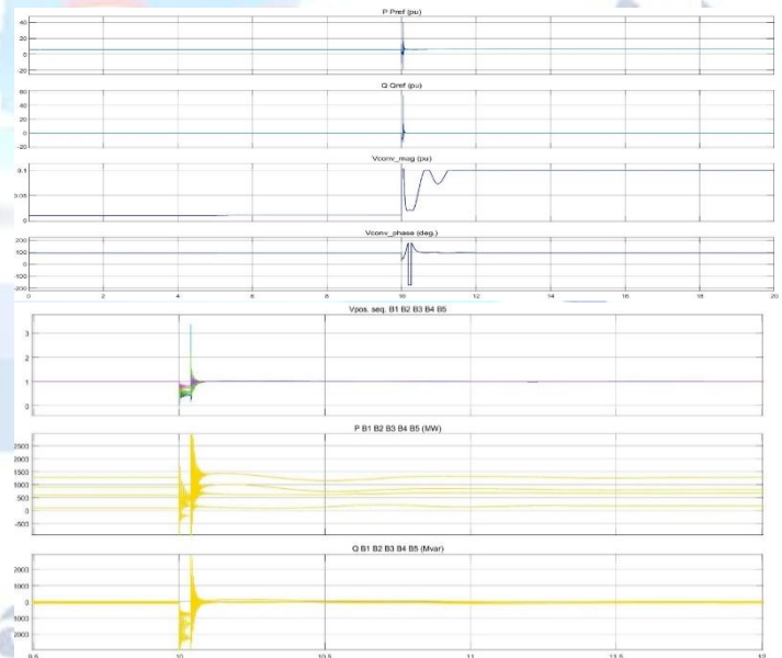
Fig .13 Simulation result of FOPIDbased UPFC
