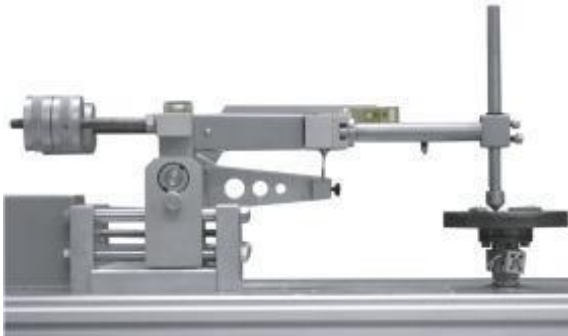
Fig.3.3. Wear performance test
