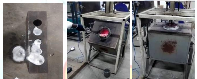
Fig.3.5. Fabrication of Hybrid composite material
