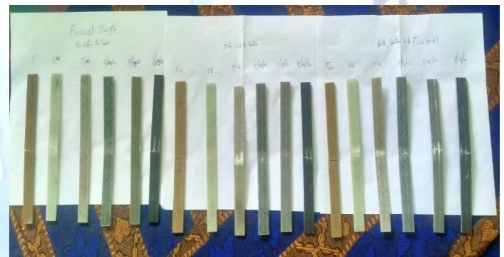
Fig:5. Tested samples of flexural strength of all specimens
