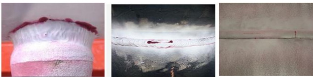
Fig-16 : Defects in LPT
