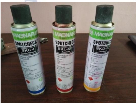
Fig-10: Developer, Pre-cleaner, Penetrant
