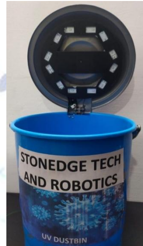
Fig 5: UVC LED's OFF when the dustbin is open in between 7.5 minutes time duration
