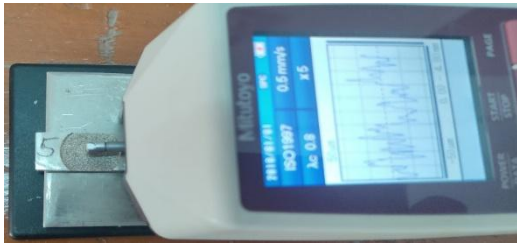
Figure 2. Surface roughness measurement by SURFTEST SJ-210
