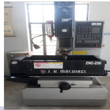
Figure 1. EDM machine set-up
