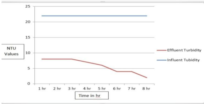
Fig 5.1.1 Graph representing Influent and Effluent Turbidity
