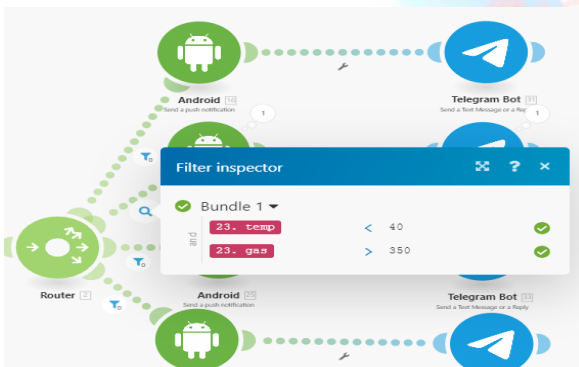
Fig. 9. Gas leakage alert is detected
