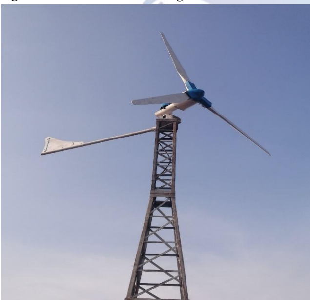
Figure 2: Final setup of PMMSG based WECS
