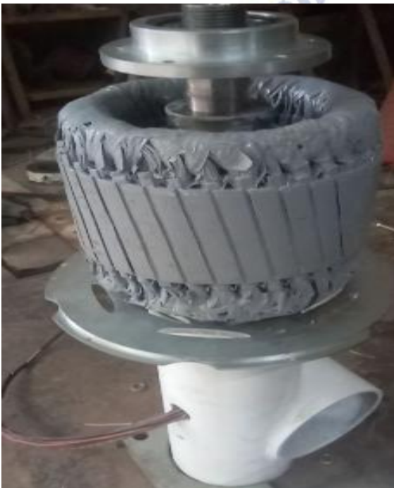
Figure 1: Front view of Redesigned PMMSG
