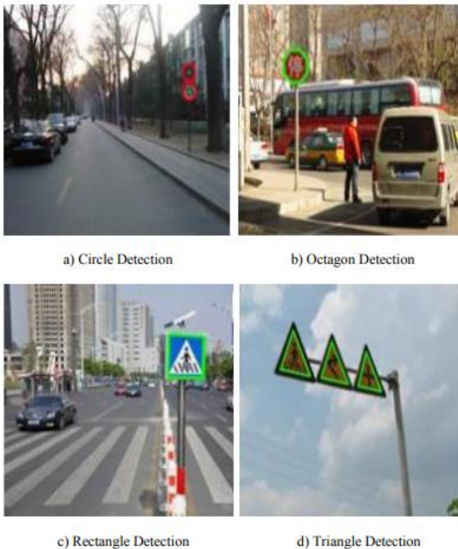
Fig. 5 Results of traffic sign detection using both color and shape information, Courtesy: [29]
