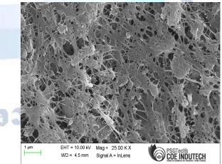
Figure 2. Surface morphology of BC sheet at 25000 X magnification
