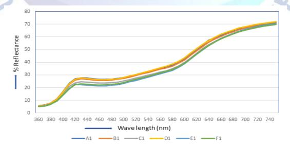
**Figure 4** Wavelength- reflectance curve of silk fabric dyed with red kidney bean extract in different acidic pH
