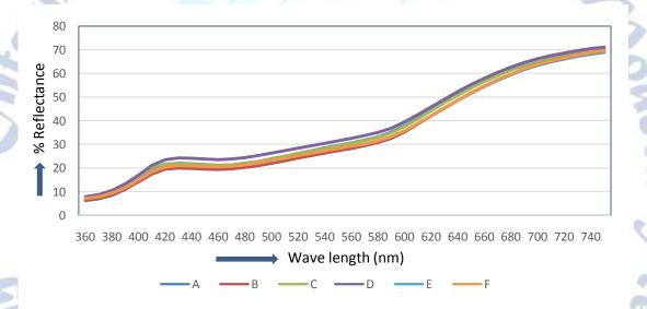
Figure 3 Wavelength- reflectance curve of silk fabric dyed with red kidney bean extract with Alum
