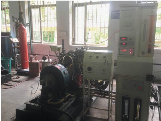
Figure 2: Pictorial View of Engine Set Up.
