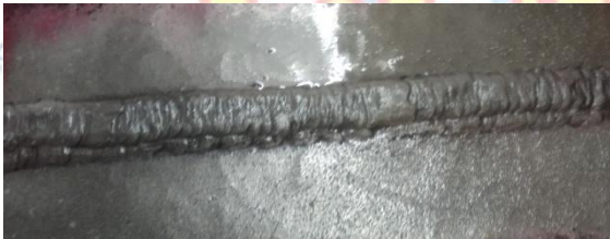
Fig6: Both the figs indicate the magnetic particle application and detecting the flaws of sub-surface
