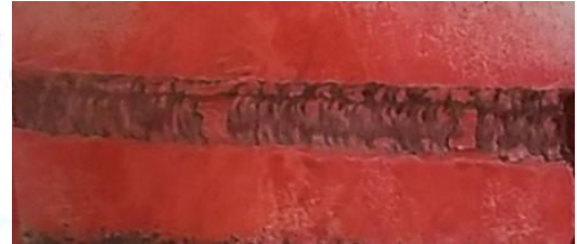
Fig 2: After the application of the penetrant
