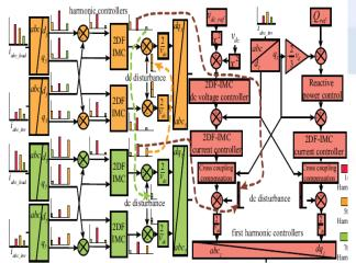
Harmonic disturbances propagation and compensation in a 2DF-IMC based filter-less SRF
