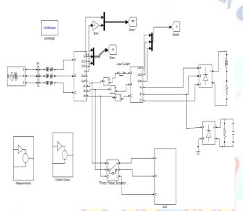
Fig.(6): Matlab/Simulink circuit for DSTATCOM model of Three Phase four Wire System
