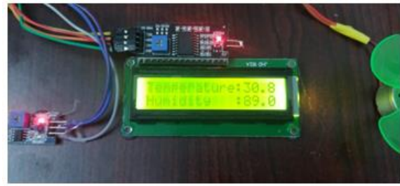
Figure.15 LCD display for temperture and humidity sensor
