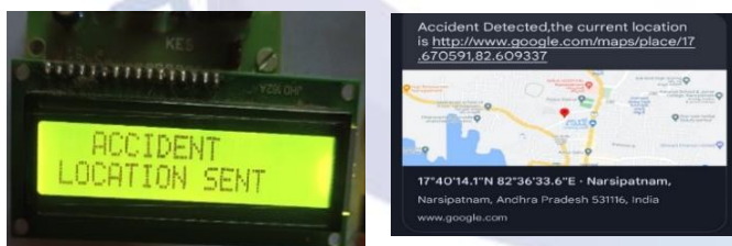
Fig.5.5 Accident Detection Results
