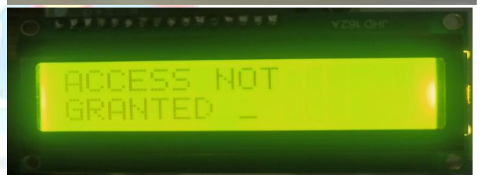
Fig Access is Not Granted so the lock will not open and the buzzer gets on, LEDs will blink
