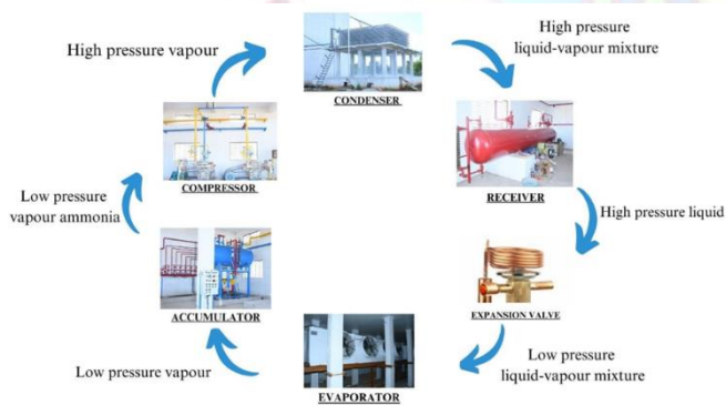
Figure 1. Refrigeration Cycle of Cold Storage Plant
