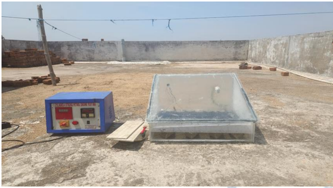
Fig 1. Final assembly of single slope solar still
