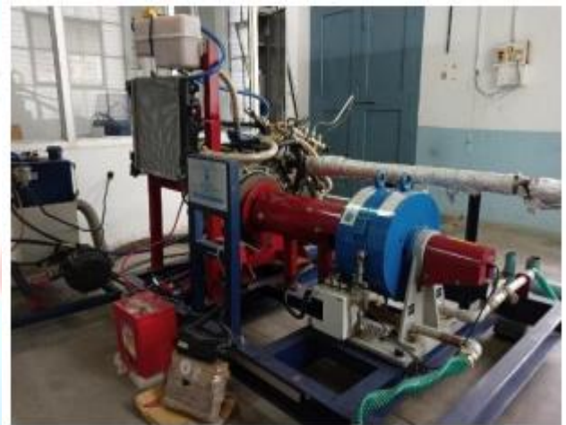
Figure 5: 4 stroke 1- cylinder diesel engine WITH EGR
