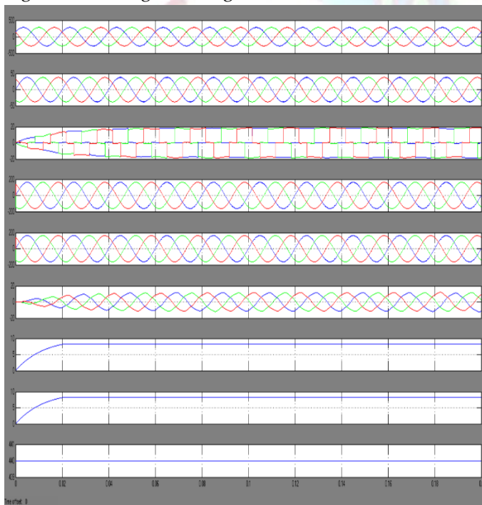
Fig: With Filter (a) Grid Voltage, (b)Grid Current, (c)Load Current, (d) Voltage at the LCL filter, (e) Voltage at PCC (f) Current at LCL filter (g) DC Voltage
