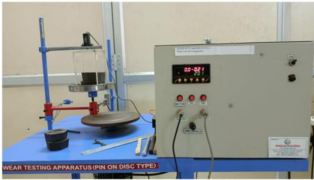
Figure :Pin on Disc Friction and wear test rig
