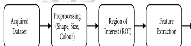
Figure 2: Preprocessing and segmentation steps for fruit detection and classification.
