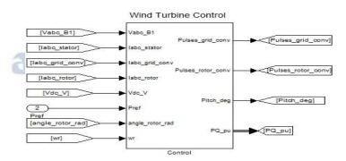
Fig 13 Control structure for Wind Turbine
