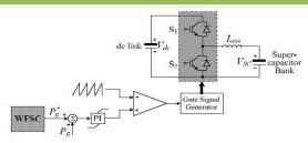
Fig 5 Configuration and control of ESS for DFIG Wind Turbine
