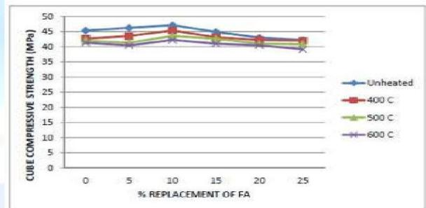
**Variations in compressive strengths at 400 °C, 500 °C, 600 °C at 56 days duration for 30 minutes**
