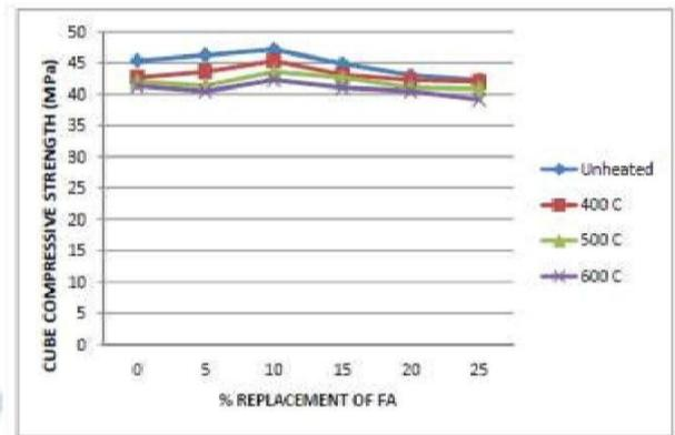
**Variations in compressive strengths at 28 days duration exposed to 400°, 500° & 600°C for 60 minutes duration.**
