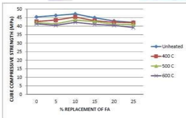
**Compressive strength of cubes when exposed to 400°C, 500°C, 600°C at 28 days for 60 minutes duration**
