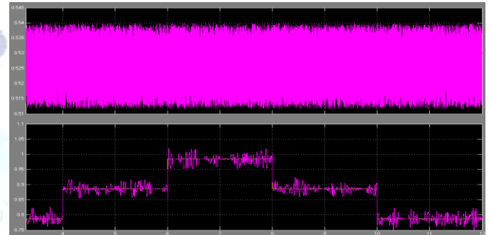
Fig. 9. Performance of the direct control scheme: (c) Flux linkage and its reference, and (d) speed reference and measured
