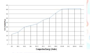
The above graph shows the variation of compaction energy w.r.t UCS.... As compaction energy increases UCS increases upto compaction energy E9 from their no significant improvement.
