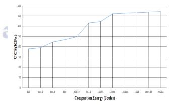
The above graph shows the variation of compaction energy w.r.t UCS.... As compaction energy increases UCS increases upto compaction energy E8 from their no significant improvement.
