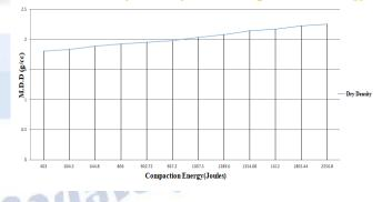
The above graph shows the variation of compaction energy w.r.t MDD.... As compaction energy increases MDD increases upto compaction energy E9 from their no significant improvement.
