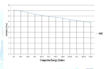
The above graph shows the variation of compaction energy w.r.t OMC.... As compaction energy increases OMC increases upto compaction energy E10 from their no significant improvement.
