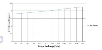
The above graph shows the variation of compaction energy w.r.t MDD.... As compaction energy increases MDD increases upto compaction energy E10 from their no significant improvement.
