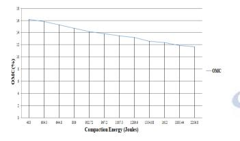
The above graph shows the variation of compaction energy w.r.t OMC.... As compaction energy increases OMC increases upto compaction energy E11 from their no significant improvement.
