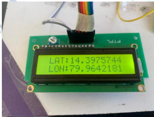
Fig 10 : LCD Showing GPS Location
