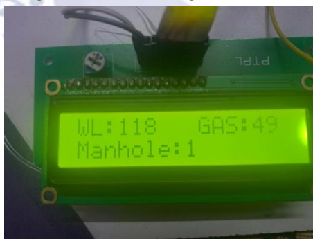
Fig 11: LCD Showing Sensor Values
