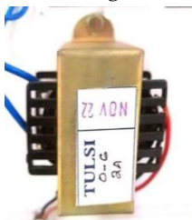
Fig:3 230V \ 6V, 2 Amps Transformer
