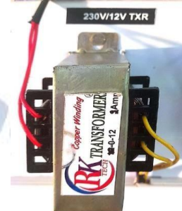
Fig:4 230V \ 12V, 2 Amps Transformer AC to DC Converter & Buck Convert
