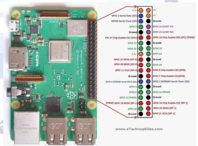
Figure 4. Pin diagram of Raspberry 3B+
