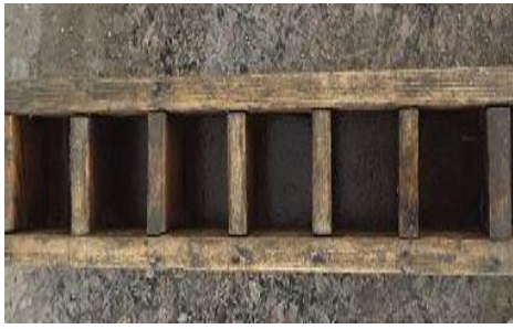
Fig 2: Moulds of Cubes of Size 50mm*50mm*50mm
