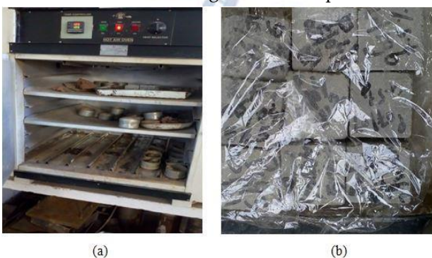
Fig.4:(a) Hot Air Oven and (b) Cubes Protected from Humid Atmosphere
