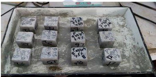
Fig. 3: Cubes Casted for Thermal Cycling Test
