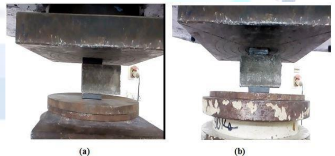
Fig 5: Different Arrangements of Bearing Plates on UTM
