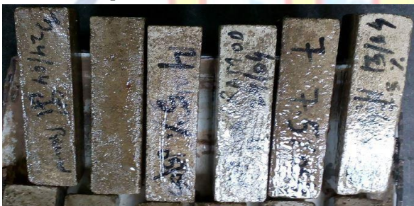
Fig 3: Prisms with Epoxy Coating
