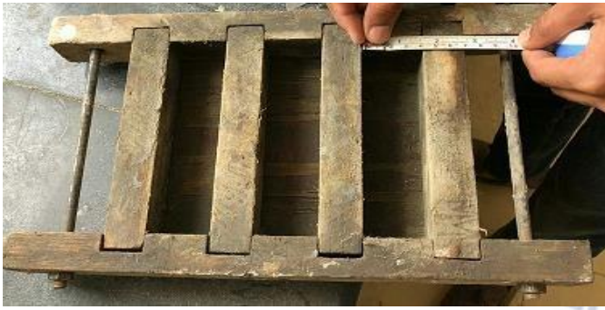
Fig 2: Moulds for Prisms of Size 40mm*40mm*160mm.
