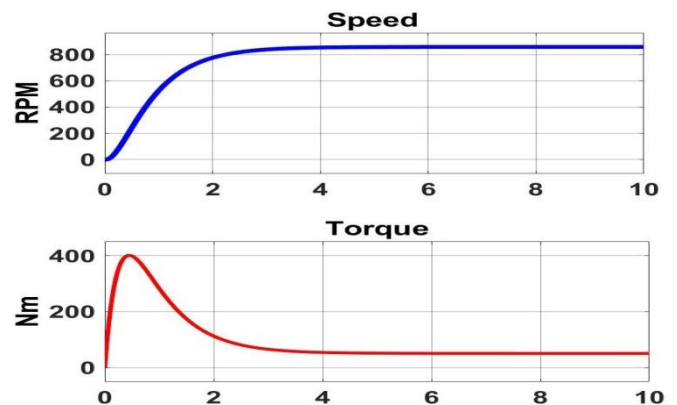
Diagram 1: with Constant Armature voltage & torque load in simulation.
