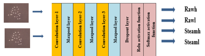
Fig - 3: Customized CNN model used for classification of rice types
