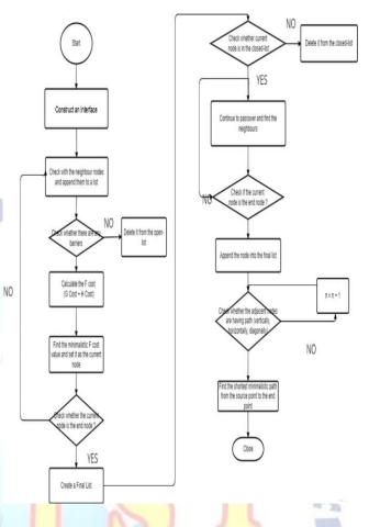
Step 5: All nodes on the close-list are evaluated once the goal point is added using the functions P(x, y) and W(x, y), and any that fail muster are removed;
