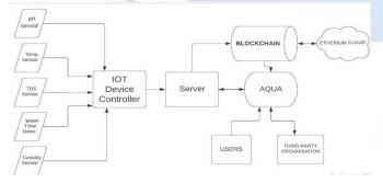
By using IoT devices to monitor the flow of water through the pipeline, it is possible to detect when there are unusual spikes or drops in flow, which could indicate a leak. This information can then be used to repair the leak and prevent further water loss.
