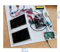
Firstly, this project proposes a solar energy measurement using raspberry pi, in which four parameters like voltage, current, temperature and light intensity is measured. These parameters where given as the input value to Arduino and then to raspberry pi and the output is displayed on 16\*2 LCD display.
