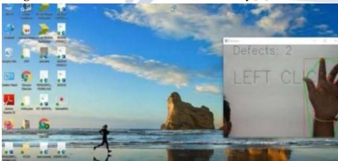
Left click operation is performed by hand gestures The above figure shows that the left click operation is performed by using the hand gesture where the number of defects is two.
