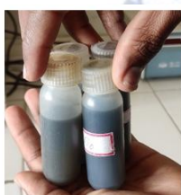
Figure 7 Iron nanoparticles solution in centrifuge vials
