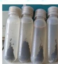
Figure 9 Particles separated after centrifugation
