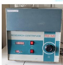
Figure 8 Centrifugation at 8000 rpm for 20 min
