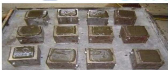
Compaction of cubes
