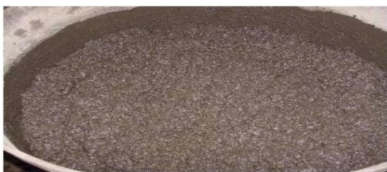
Fresh Geo polymer concrete
