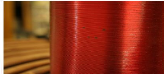
Fig.13 Results of inadequate space between the coils: arcing between the two occurred, burning the secondary coil at several points.
