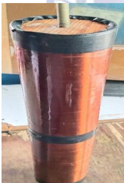
Fig.12 Secondary Coil used in the Tesla Coil paper
