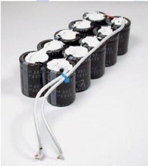
As the name implies, a capacitor bank is just a collection of capacitors of the same rating. Capacitor banks can be connected in series or parallel, depending on the required rating. Individually and in banks, capacitors are used to store and condition electrical energy.
