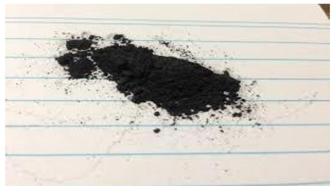
Aluminum powder of 50µm size are mixed with B4C and aluminum powder and B4C and graphite mixed in above given table powders are prepared.
