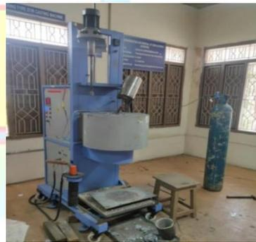
Fig 2 Stir Casting Equipment
