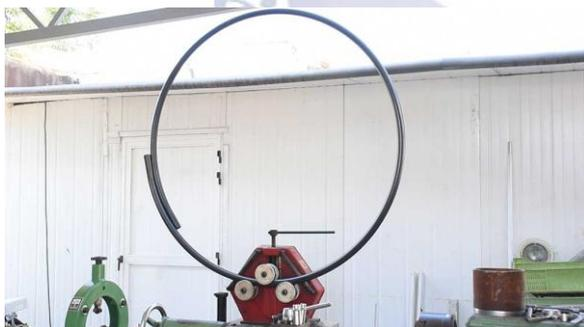
Fig 3. Construction of outer wheel
