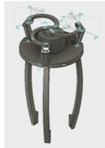
Fig 1 Initial CAD model of Link operated gripper.
