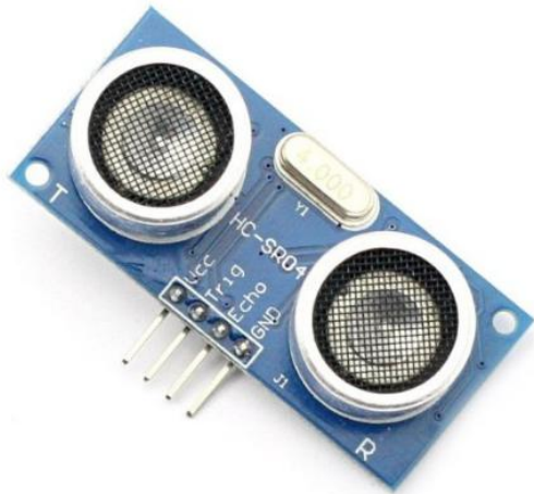
Figure: 3.3 Ultrasonic Sensors
