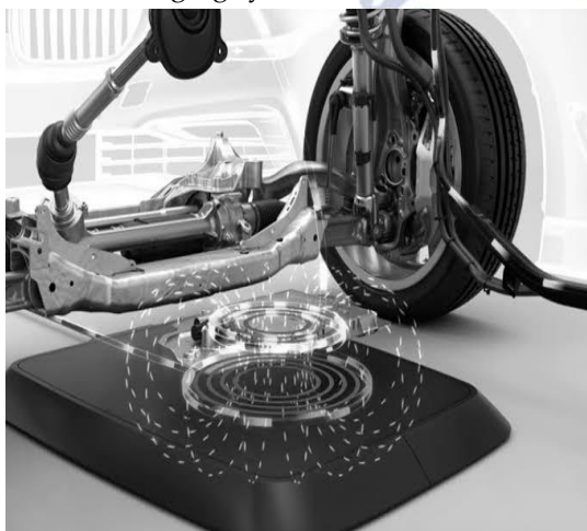
Figure : 2.1 Wire Less Charging System
